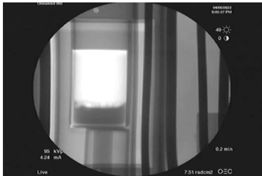
Fig. 4: Melting of H-DRI in slag heated at 1600 °C
