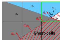
VOF extrapolation with contact angle
