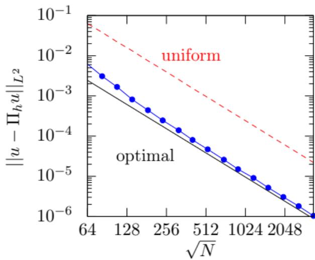
Interpolation errors only (injecting  $u$  on nodes)
