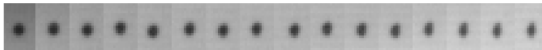
Fig. A1 Case 1249 droplet deformation evolution: airfoil velocity = 90 m/s, chord size = 690 mm, and droplet radius = 181 \mu\text{m} .
