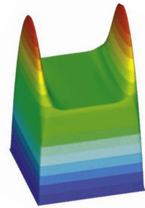
3. MHD flows in conducted duct
