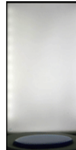
A puddle jumps from superhydrophobic surface in low-g condition.
