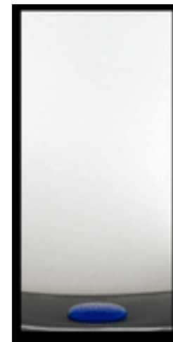
A puddle jumps from superhydrophobic surface in low-g condition.
